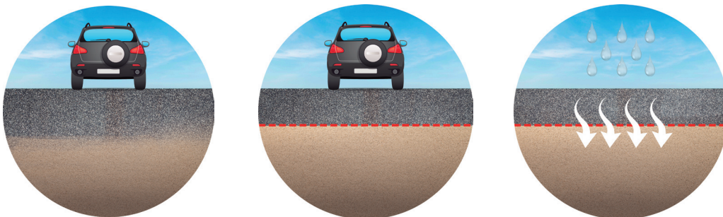
With and without separation and filtration geotextile
