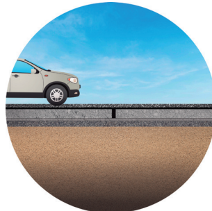
Rigid pavement rehabilitation with asphalt overlay
