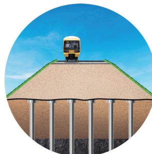
Embankment on piles
